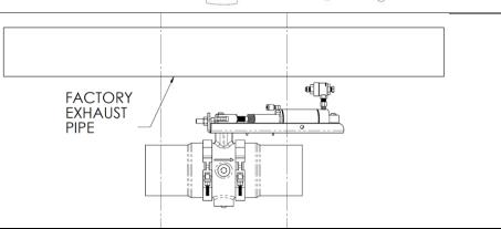
Disassemble the exhaust pipe adapters from the brake valve and slide one of them on the front exhaust pipe. Fully weld this to the pipe to create a complete seal.
