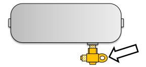
If the air tank has a spare 1/8"NPT outlet fitting install here. Otherwise the installer will have to supply fittings to allow for a 1/8"NPT fitting to be installed.
