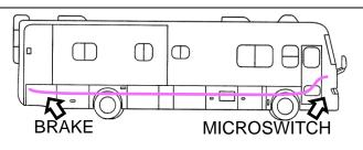
WITH AIR COMPRESSOR ONLY Connect the PINK wire to the PINK wire from the air solenoid/regulator kits PINK wire. Use the pre-installed heat shrinkable butt connector. Crimp the connection then use a heat gun to seal the connection.
