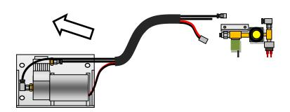
Thread in the supplied "pancake" air filter to the fitting on the air suction line. Zip tie this filter in the engine compartment in a clean dry location.
