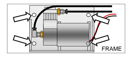
Four self-threading screws and four washers (1500369 and 1500367) have been provided which may be used for direct frame mounting. If using these fasteners, mock up the pump assembly to the frame and scribe the four holes thru to the frame. These will be the drill locations. Use a center punch to make a dimple, and then drill a 1/8" pilot hole. Now drill the final 21/64" holes. Install the bolts with a 9/16" socket and air ratchet.
