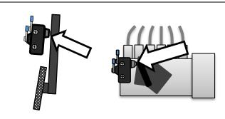
Run the remaining red wire from the toggle switch to the micro switch and crimp it to one of the switch terminals.
