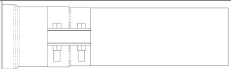
Clamp the exhaust brake assembly between the two flanges with the Marmon clamps. Align brake valve to pipes and so that it is clear of vehicle obstructions. Tighten clamps.
