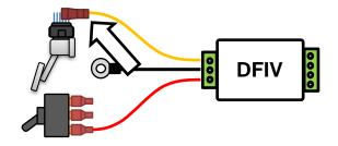
Locate the PINK wire supplied with the DFIV kit, install the end of this wire in the terminal labelled BRAKE, this is the 12v output to the exhaust brake air solenoid. Route this wire to the location that the air regulator/solenoid is installed in the engine bay.
