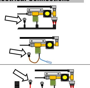
Leave the small PINK or BLUE wire for now, this will be connected to the output of the DFIV or micro switch in the following sections.
