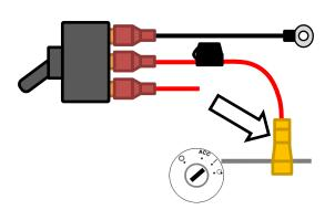
**CAUTION** Only probe ignition switch or fuse box wires. Ensure to avoid possible contact with airbag or sensor wiring.
