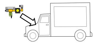
Mount the air pressure regulator/solenoid assembly using two self-tapping screws provided (1300529) or by other secure means.
