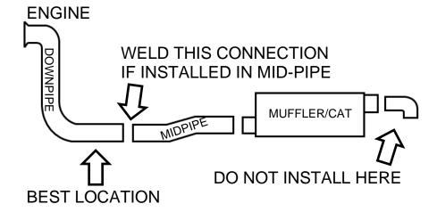
Loosely assemble the exhaust brake casting to the supplied front pipe and rear adapter pipe and mock up the area it will be installed in. Ensure the brake valve actuator will not interfere with vehicle components.
